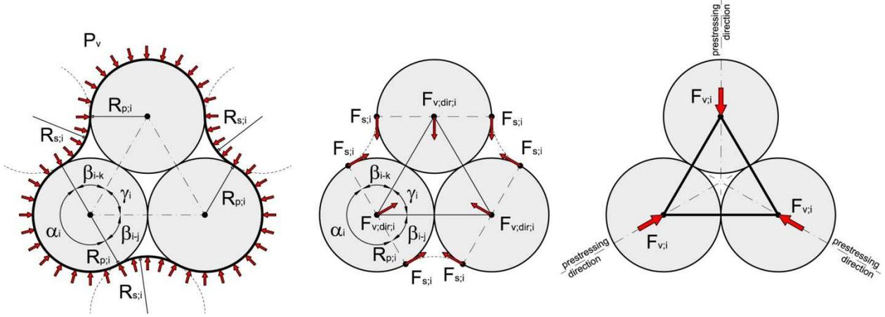
Fig. 2: vacuum pressure (a), prestressing components (b) and prestressing forces (c)
