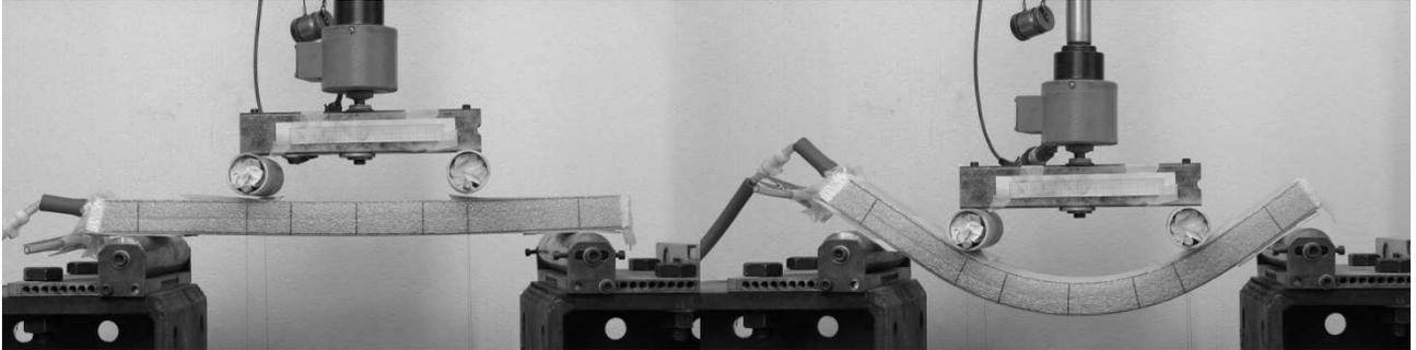
Fig. 1: bending test on a beam-shaped Vacuumatics specimen
